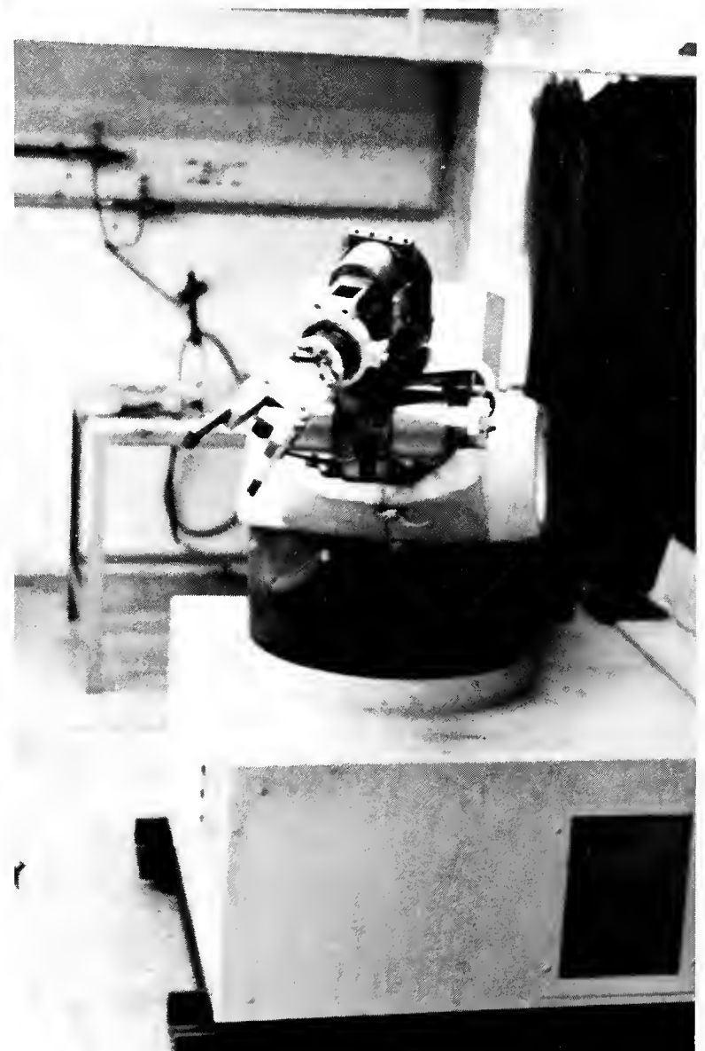
THE LONG ARM OF THE LAW —Memphis State's Unimate robot has a moveable arm that can lift several hundred pounds; however, the robot itself is stationary.
